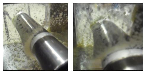
Figure 7-7: Deposition morphology on round and elliptical tubes.  $T - T_g^*$  conditions are 52.6 °C (left) and 54.8 °C. Photographs were taken at the end of the test.
