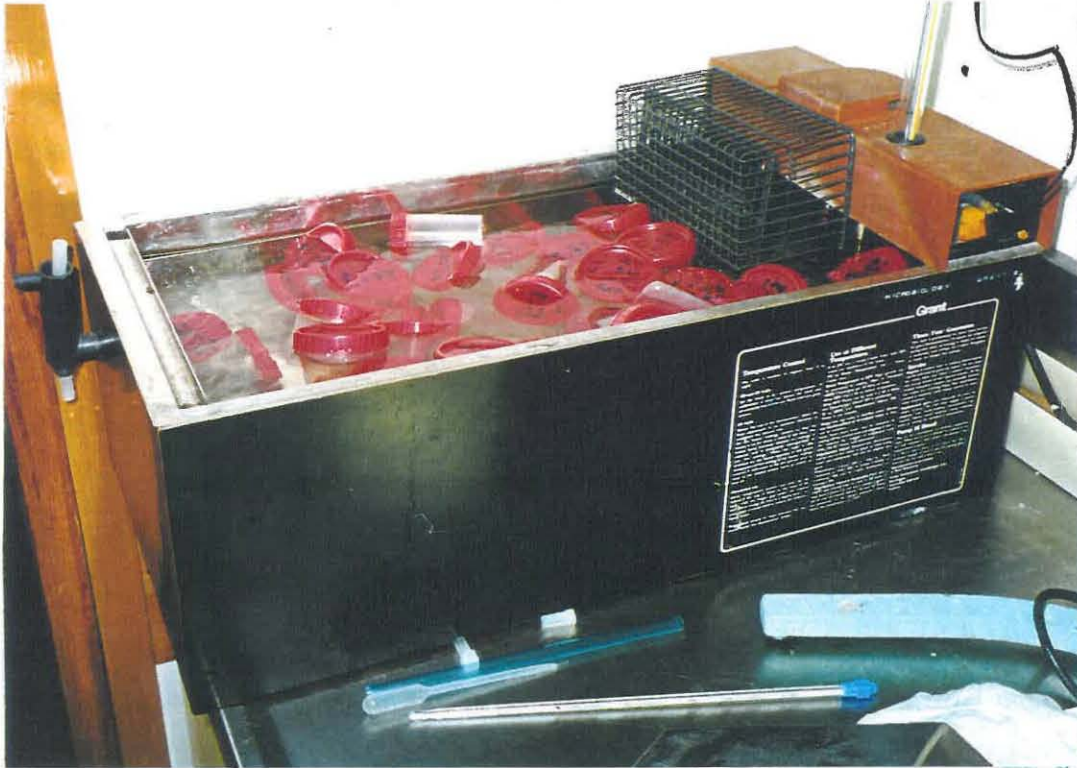
Figure 3.2: Photo of 20°C water bath with containers used in the transporting experiment.
