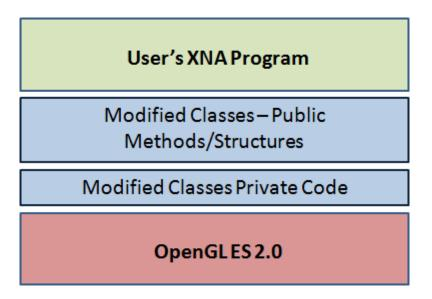
Figure.17 Architecture of Modified System on Raspberry Pi
