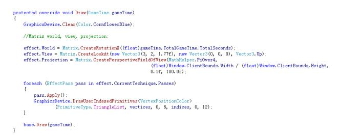
Figure.90 Draw Method for Displaying a Colored Rotating Cube with XNA on Windows
