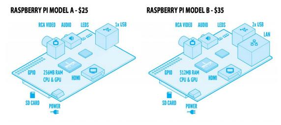
Figure.3 Layout of the Raspberry Pi [2]
