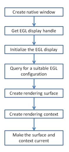
Figure.21 Process of Initialization (Setup Function)
