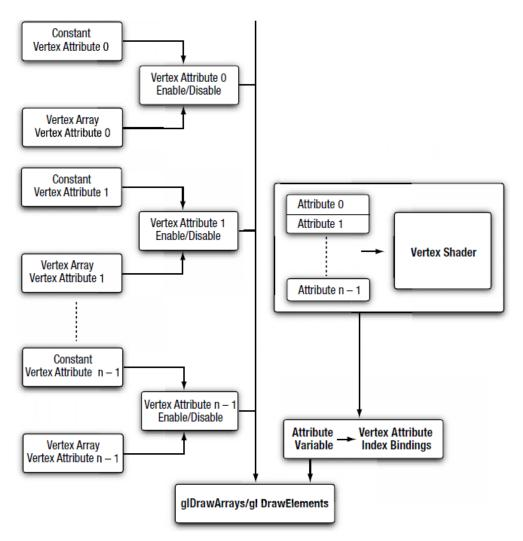
Figure.28 Specifying and Binding Vertex Attributes for Drawing Primitives
