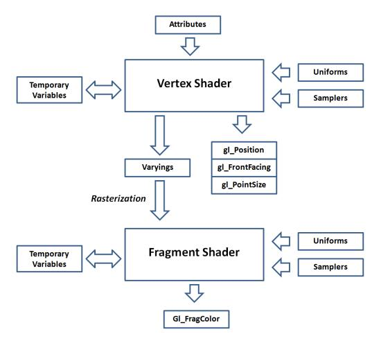
Figure.15 Inputs and Outputs of the Shaders [17]
