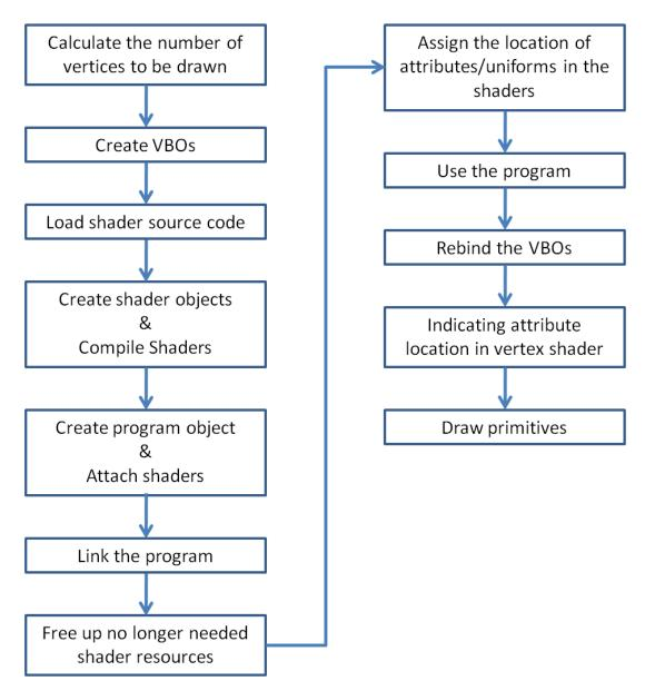
Figure.81 Process of the DrawUserPrimitives Method
