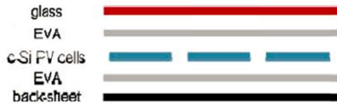
Figure 6 Schematic representation of the encapsulation of PV cells using EVA [11].
