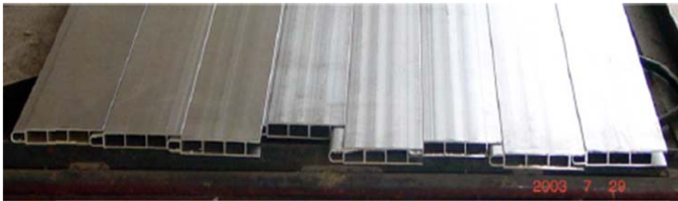
Figure 10 Flat box channels assembled to create an absorber for a PVT collector [49].
