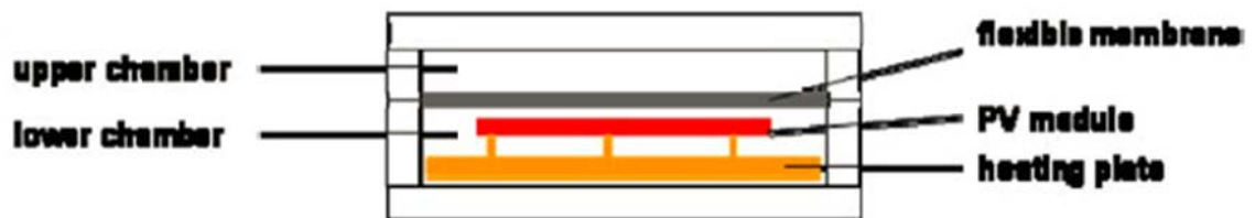
Figure 7 Flatbed laminator used to cure the EVA and encapsulate the sandwich assembly [11].
