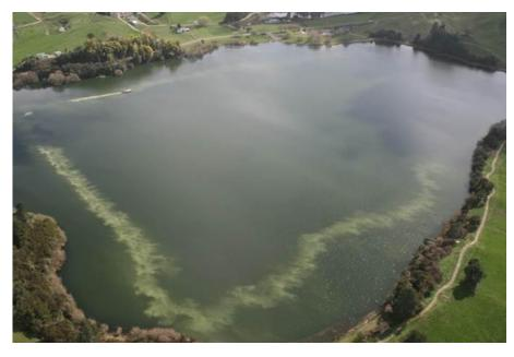
Figure 11 Aerial view of Aqual-P (modified zeolite) application in Lake Okaro, Bay of Plenty (Photo: Andy Bruere).
