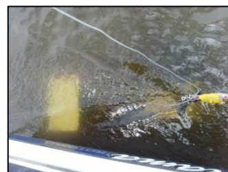
Photographs 6 and 7 BioFish instrument deployed in Lake Rotorua outside (left) and within (right) the apparent path of the Ngongotaha Stream inflow, December 2011
