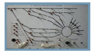
Figure 2.2: Traditional analogue controller with a block system. Switches route power to divided sections of track. [4]
