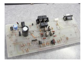
Figure 4.16: First prototype based on hardware version 1.8.
