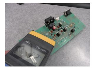
Figure 4.8: The source of the heat is confirmed and located at high side drive P-channel MOSFET of H-bridge.
