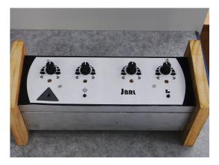
Figure 3.2: Mock-up of the enclosure for presentation to branding and software groups.
