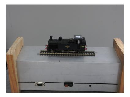
Figure 3.4: The automatic programming track activated by inversion of the enclosure.
