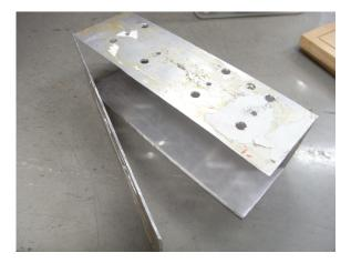
Figure 4.18: Separated rear plate of case.
