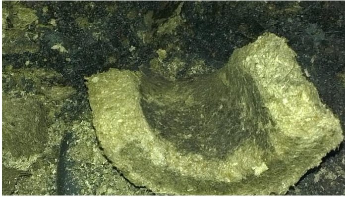
Figure 50. Dry compacted sawdust prior to decomposition, bulk density 1,202 kg/m 3 .
