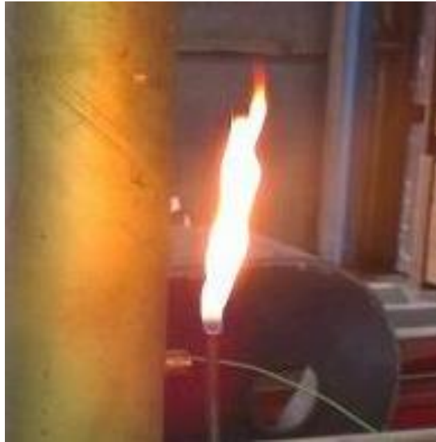
Figure 4. Syngas flare from Lakeland Steel's pilot plant processing green sawdust.
