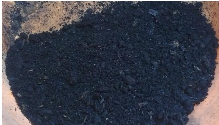
Figure 2. Char produced from Pinus Radiatta sawdust using Lakeland Steel Ltd.'s pilot plant.
