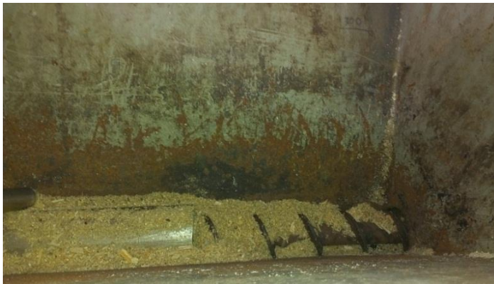
Figure 49. Loose sawdust being fed through bulk density 280 \text{ kg/m}^3 .
