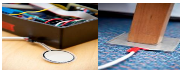
Figure1: Wireless sensing units monitoring a subject bed usage.
