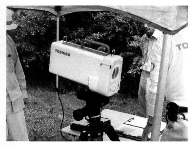
Fig. 1. The Toshiba "Gamma Camera" (under shade cover because of hot, bright sunny weather). (Lowe)
