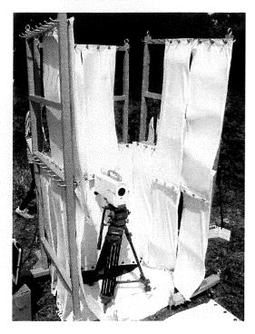
Fig. 5. Gamma camera set up in a laboratory situation indoors with full lead shielding in the white 'sheets' hanging alongside and placed beneath the camera. Note also 10-kg lead blocks right next to the camera itself. (Lowe)
