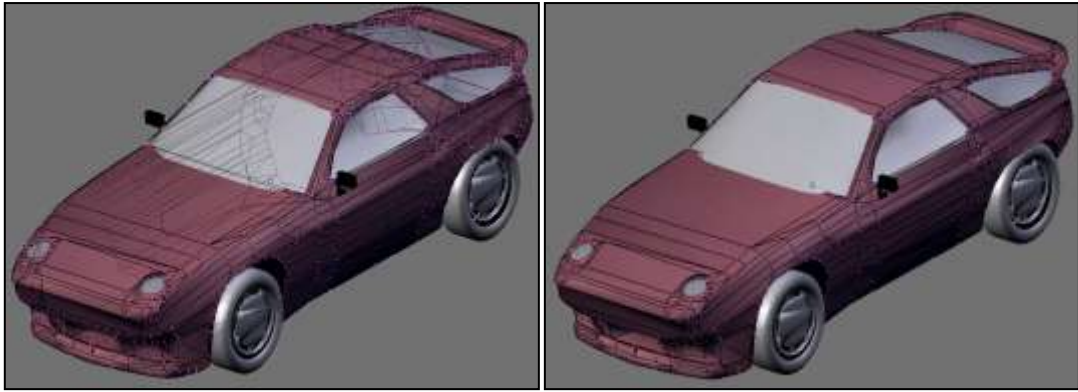
Figure 5.8: The model of a car: (left) without back surface removal and (right) with back surface removal
