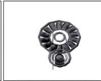
Figure 3. After both fans are aligned horizontally and vertically. View of rear fan from behind. Showing front fan almost completely obscured
