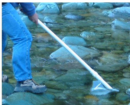
Figure 2. Deployment of the Hicks handle net for sampling algal drift.
