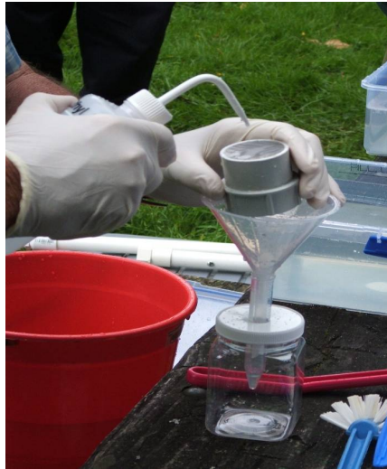
Figure 3. Wash the material from the cod end into the Falcon tube with 70% ethanol.
