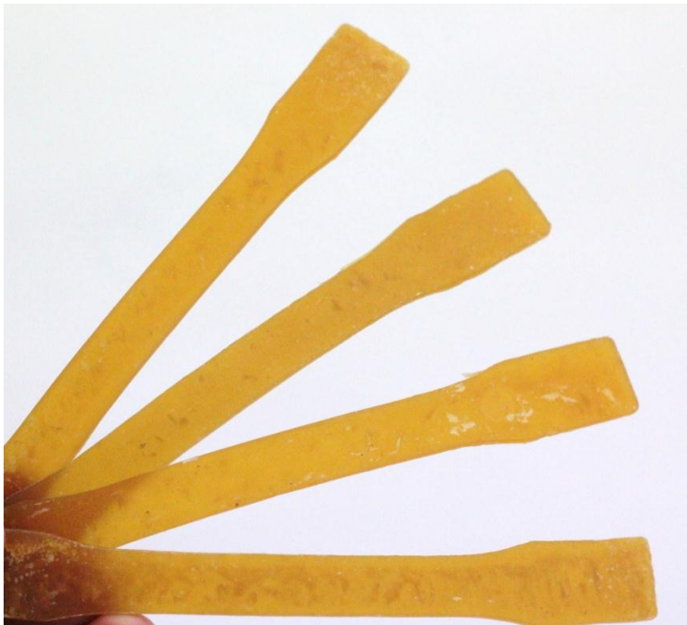
Injection moulded samples produced using peracetic acid treated bloodmeal.
