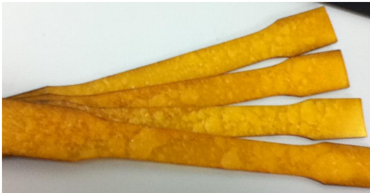
Figure 80: Compression moulded 3 % PAA treated bloodmeal cut into dog bone tensile bar samples.
