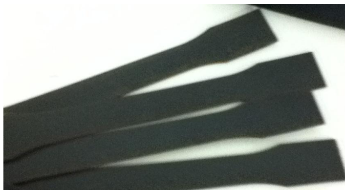
Figure 81: Compression moulded 1 % PAA treated bloodmeal cut into dog bone tensile bar samples.
