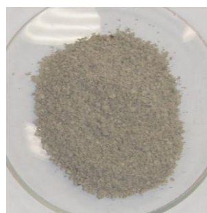
Figure 26: Sodium hypochlorite (15%) treated RBCC.
