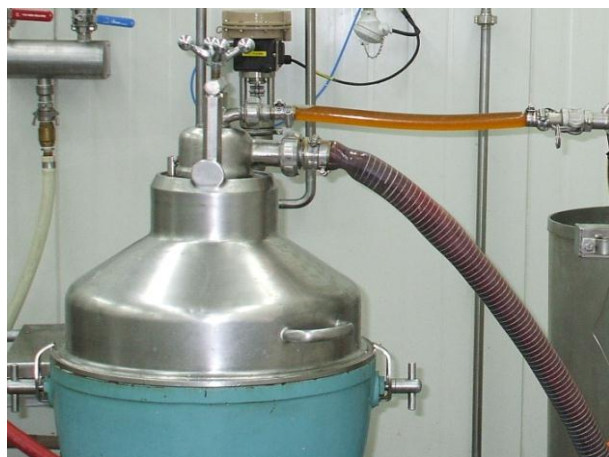
Figure 2: Blood being centrifuged into plasma (orange) and RBCC (red).
