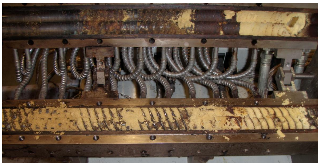
Figure 78: Failed attempt at extruding sodium chlorite treated BM.
