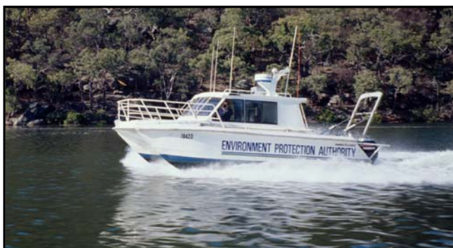
Figure 3.1 The 8.5m twin hulled RV Glaucus used for routine Port Hacking sampling, Niskin, CTD and ADCP profiling.
