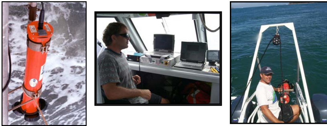
Figure 3.5 RDI 300KHz profiling ADCP (left), deployment (right), and operation (centre).
