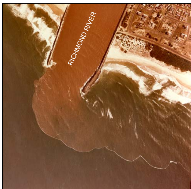
Figure 7.13 Trained entrance of the Richmond River at Ballina illustrating wave structures and turbulence along the seaward front of the river plume. OEH Aerial Photogram 13/5/83.
