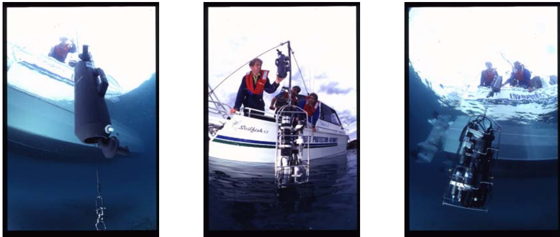
Figure 3.9 Niskin (left) and CTD (right) vertical profile system (centre)
