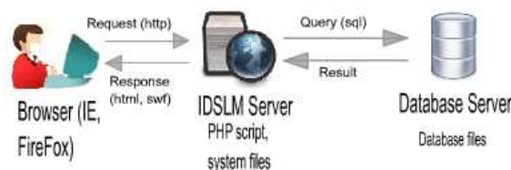
Figure 5.1: Power and energy online system architecture.
