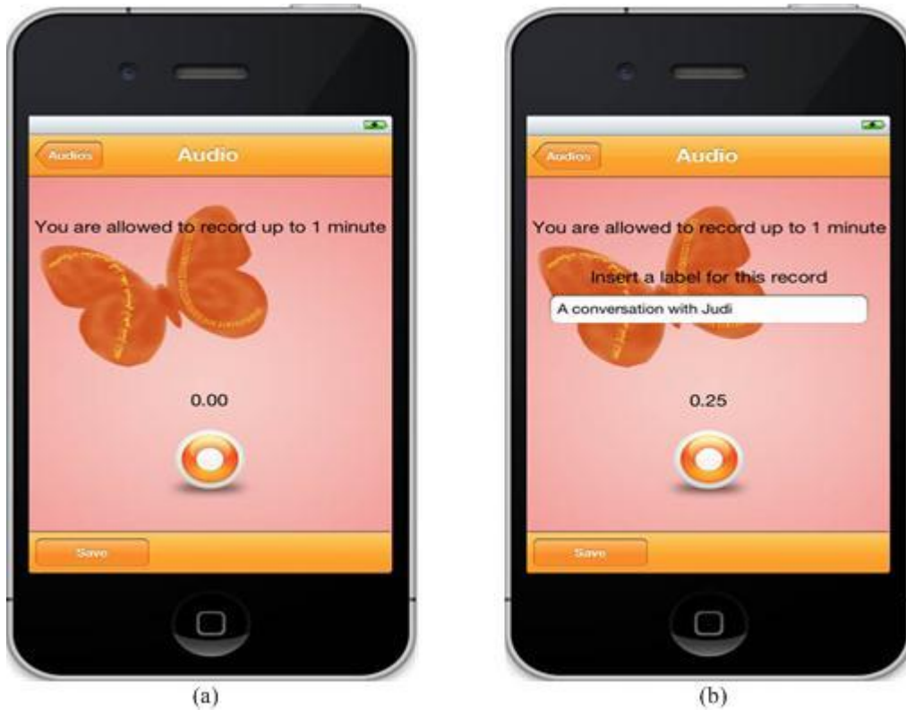
Figure 5.20: (a) The Audio window allows the user to record the target moment and it includes an instruction of the maximum length of the recorded audio. (b) When the user stops recording, the user is allowed inserting a caption of the recorded audio.
