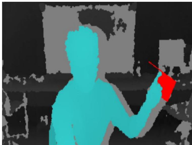
Figure 28: Depth image showing the finger search algorithm in action
