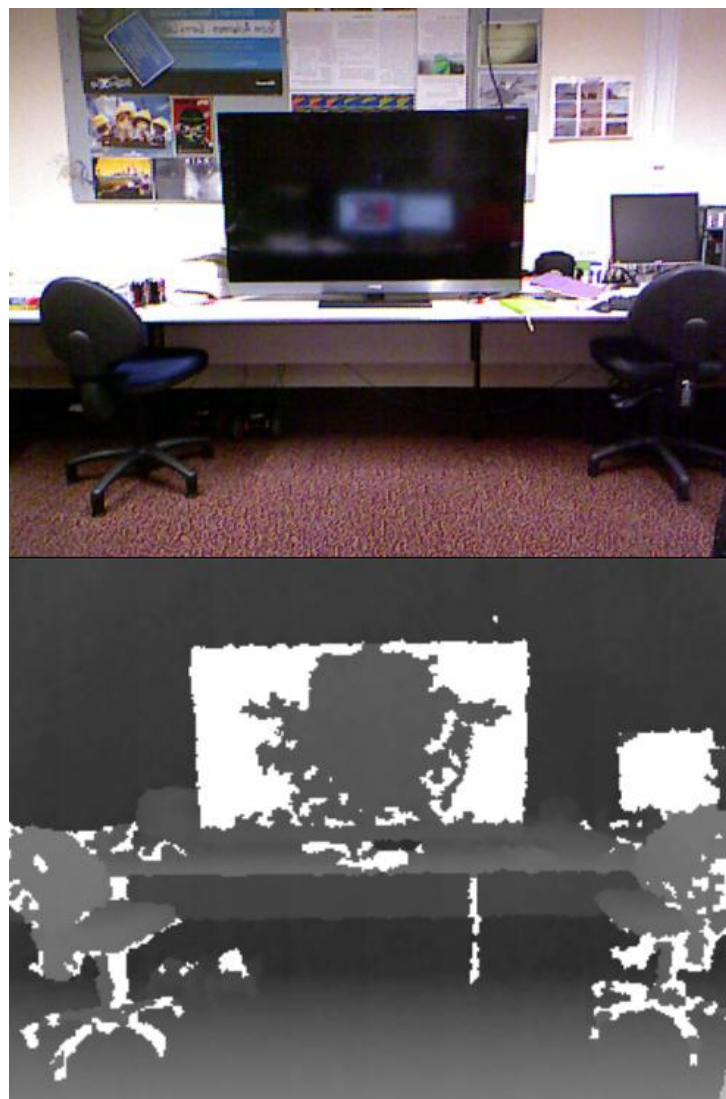
Figure 31: The bottom image is the TV screen as seen by the Kinect's depth camera, the top images is the same scene as seen by the Kinect's colour camera.
