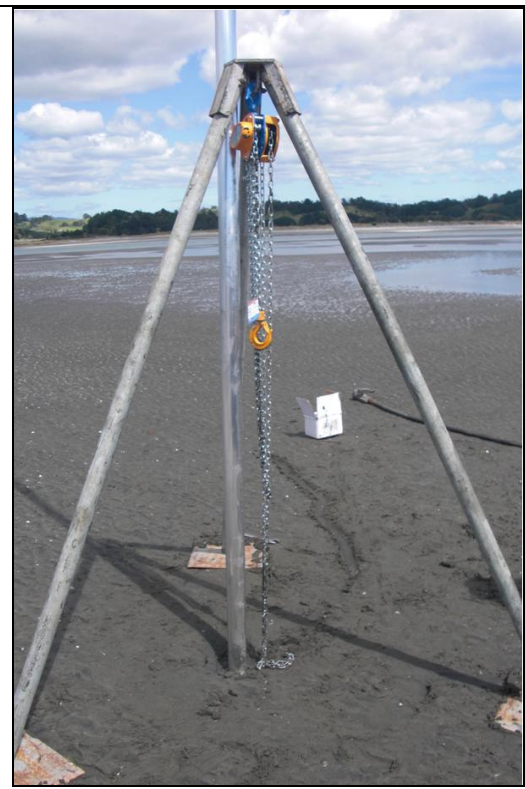
Figure 3.2 Block and Tackle lifting rig for recovering the core
