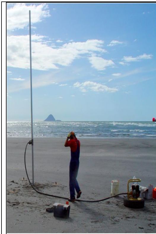
Figure 3.1 Vibrocore tube clamped to motor
