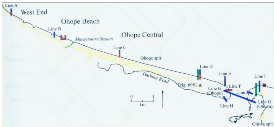
Figure 2.6 Survey lines used to measure rates of erosion and accretion at Ohope and Ohiwa Spits. Green, Gibb (1977); red, Richmond et al. (1984); brown, Hodges and Deely (1997); blue, Murdoch (2005).
