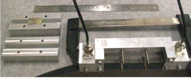
Fig. 3. Picture of the scale model with interchangeable clamshell parts for calibration visible alongside.
