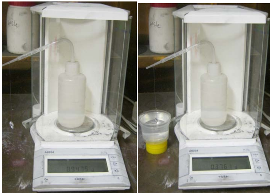
Figure 3.3: The set up used for the density measurement
