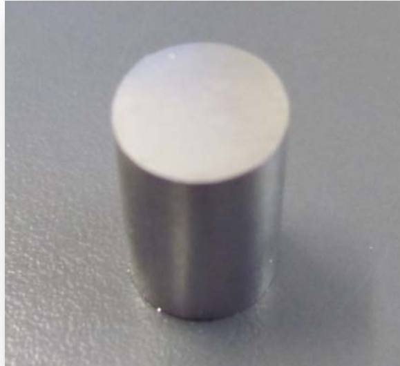
Figure 5.2: Picture of compression testing sample
