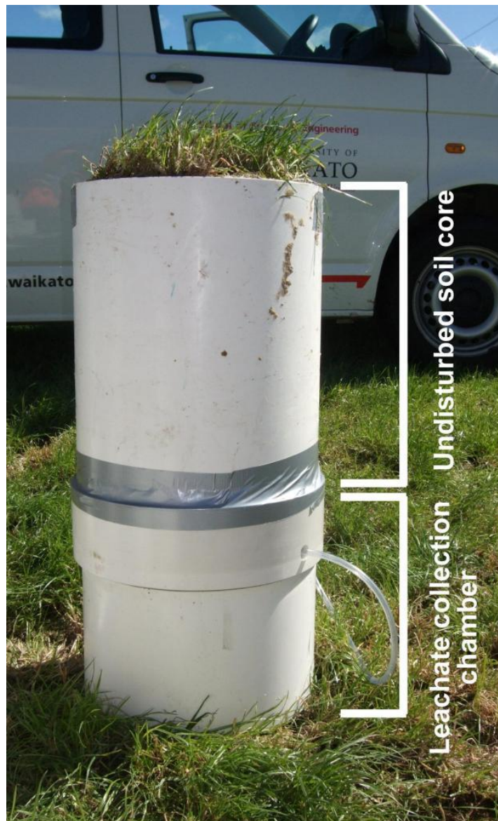
Figure 3.5. Lysimeter prior to installation. Note PVC tube exiting leachate collection chamber for sampling purposes.
