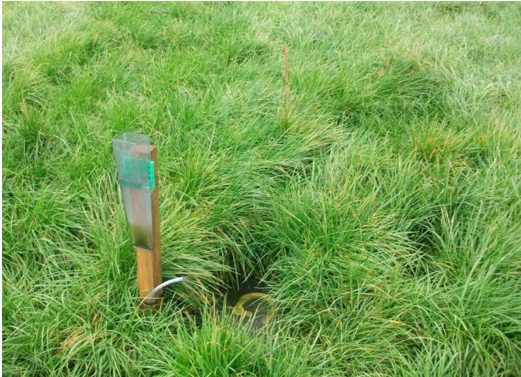
Figure 3.3. Installation of a lysimeter in the field. A plastic rain gauge with sampling tube attached is visible in the left foreground, and just visible to its right is a 0.4 x 0.4 m concrete paver. Visible in the middle ground is a bamboo stake identifying the edge of a lysimeter.
