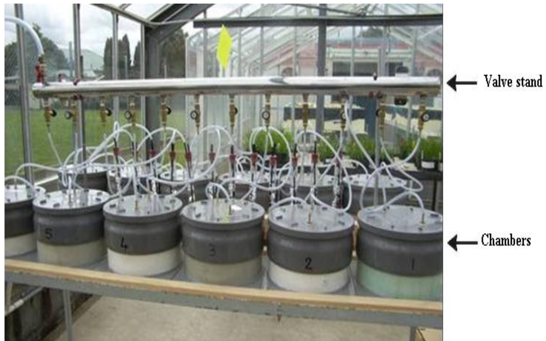
Figure 3.1 Chambers used to measure ammonia emissions from urea applied to soil (Figure from Bolan et al. , 2004a)
