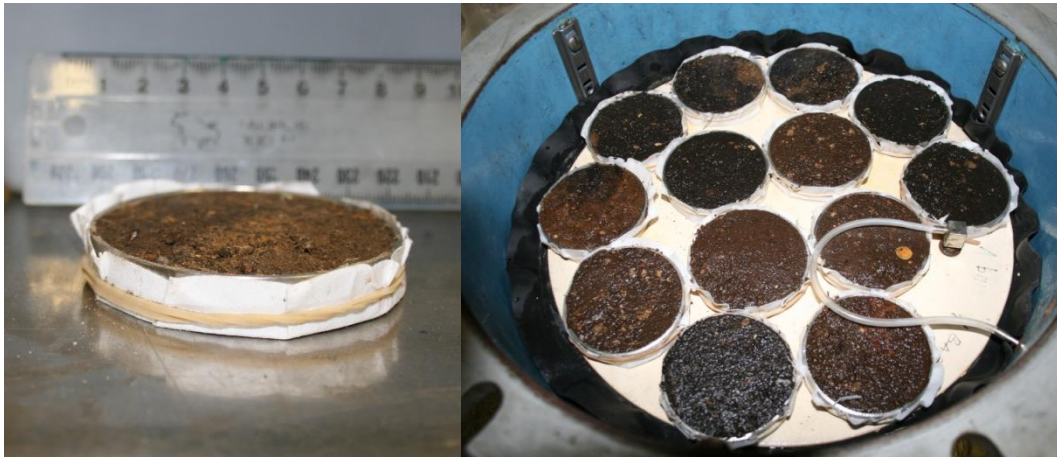
Figure 4.8 Samples for moisture retention measurement on pressure plate apparatus a: Individual sample; b: set of samples water saturated sitting on porous ceramic plate inside extraction vessel
