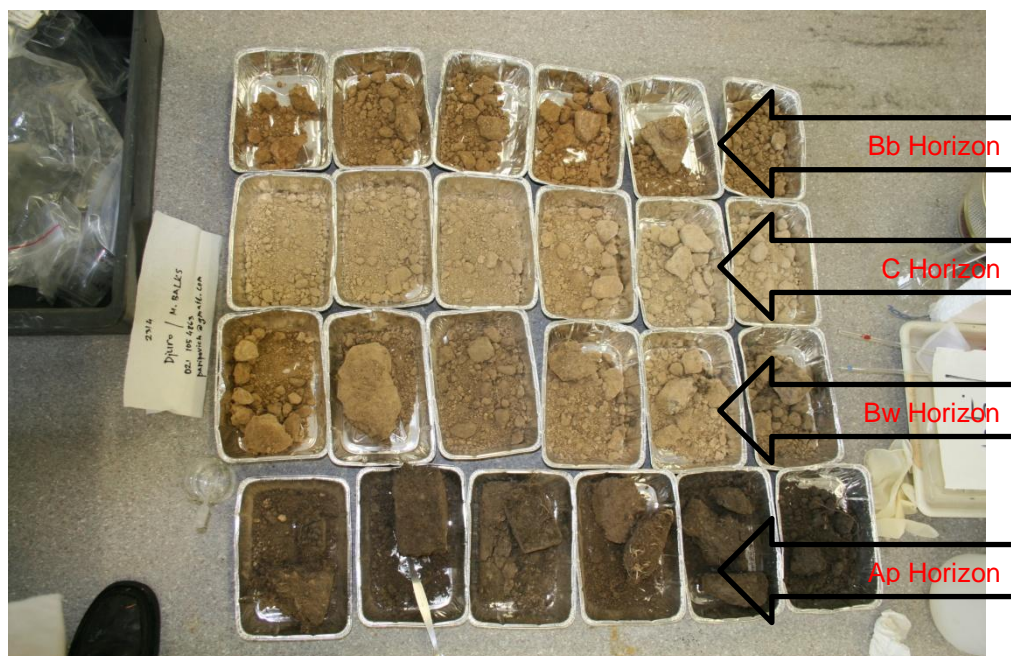
Figure 4.6 Air dried soil samples from Tokoroa prepared for water repellency determination in the laboratory
