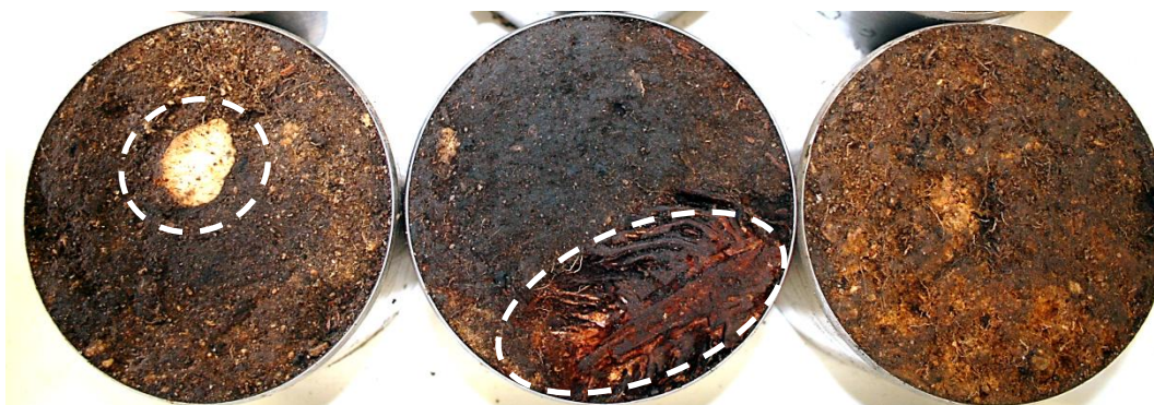
Figure 7.1 Undisturbed soil cores used for hydraulic conductivity and soil dry bulk density measurement.
