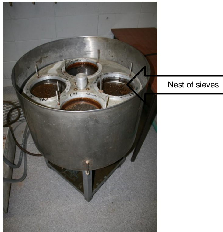
Figure 4.7 Equipment used for the aggregate stability determination in the laboratory
