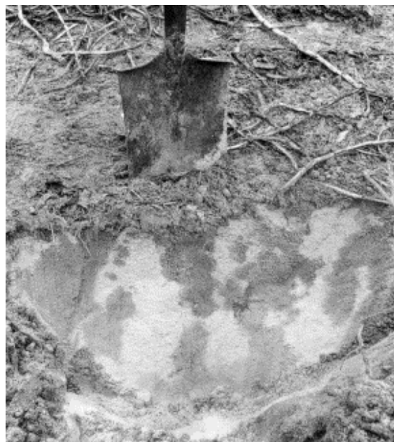
Figure 2.3 Uneven wetting patterns caused by water repellency in sandy soil near Geraldton, Western Australia, following a large rainfall event (75 mm in 3–4 h in March 1999), (from Doerr et al. 2000).
