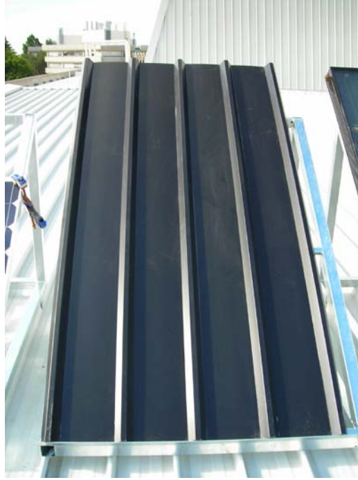
Fig. 3 Prototype building integrated solar collector
