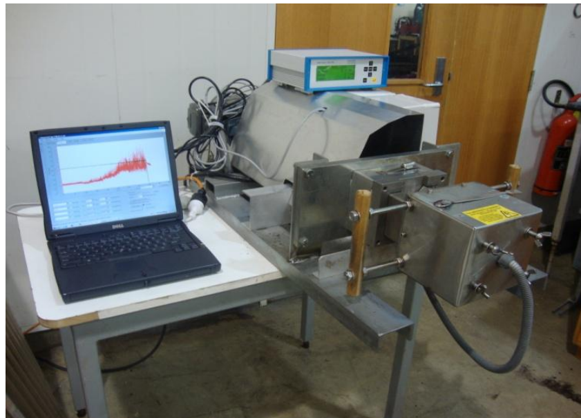
Figure 49: Batch mixer equipped with torque sensor
