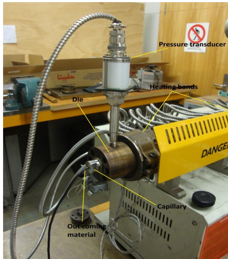
Figure 44: Capillary setup
