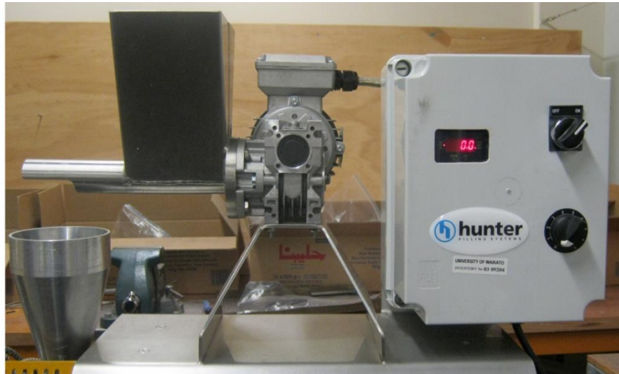
Figure 46: Feeder with control
