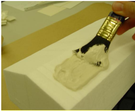
Figure 2.9 Coating the mold with white GIB compound
