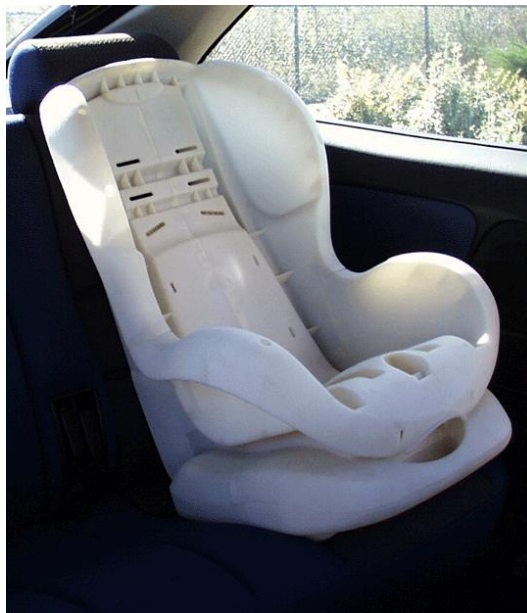
Figure 5.11 Thermoplastic SLS part (source ENME480)
