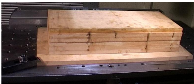
Figure 5.16 MDF block clamped to table for machining
