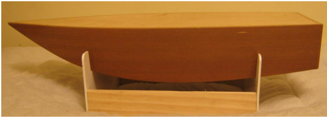
Figure 5.18 Mold sanded and coated with varnish
