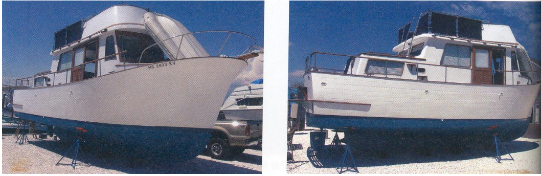
Figure 3.14: A semi-displacement hull (Sweet, 2007)
