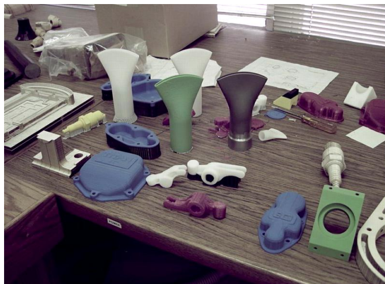
Figure 5.9 Parts made by FDM (source: ENME480)
