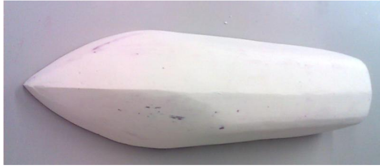
Figure 2.12: A finished mold ready for vacuum forming
