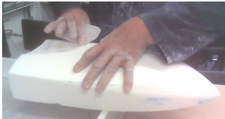
Figure 2.11 Sanding the mold for finishing
