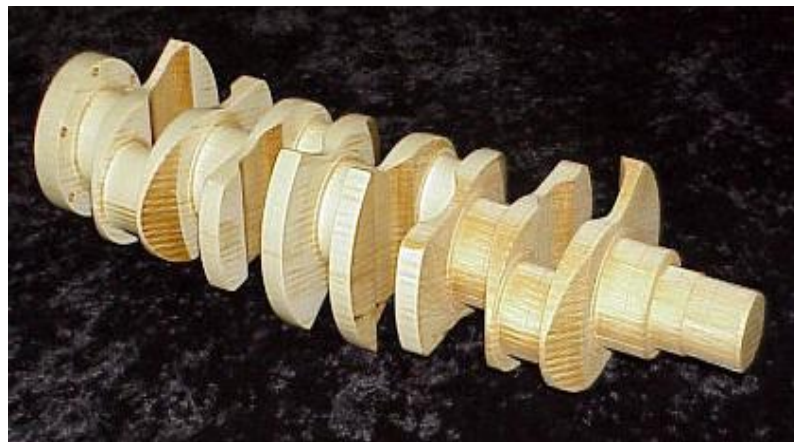
Figure 5.7 A crankshaft fabricated on LOM (source: ENME480)
