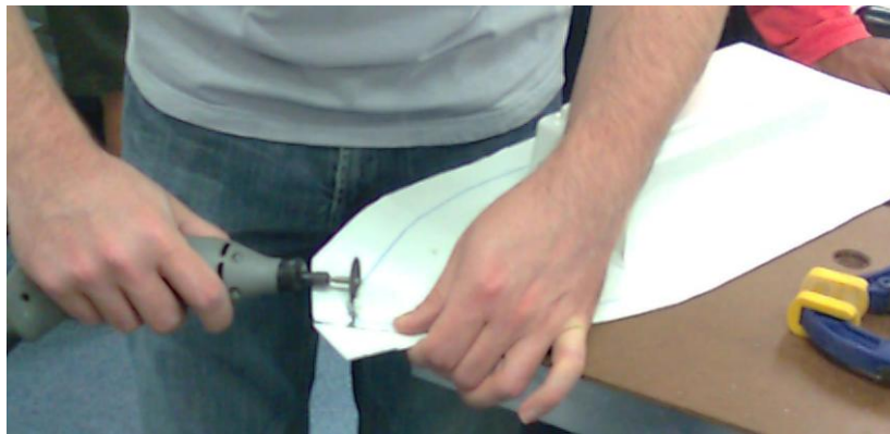
Figure 2.3 Using a power tool to trim the deck
