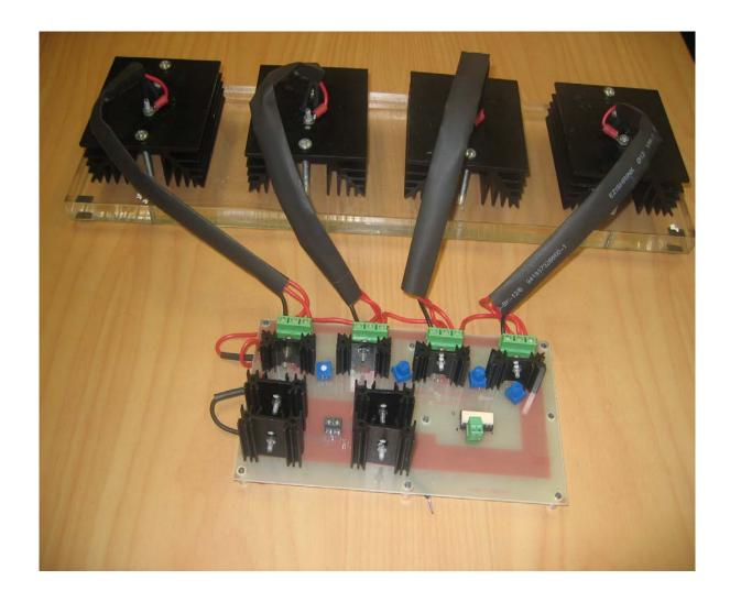
Figure B.2: Photograph of Transistor array
