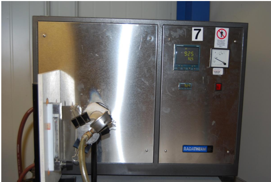
Figure 4.17: Tubular Vacuum Furnace used for the heat treatment
