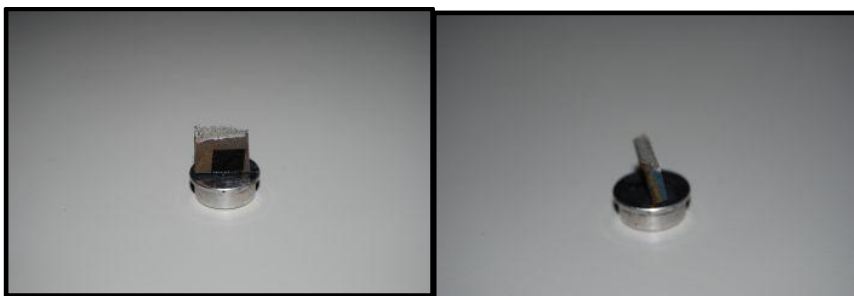
Figure 4.13: Fracture surface for SEM
