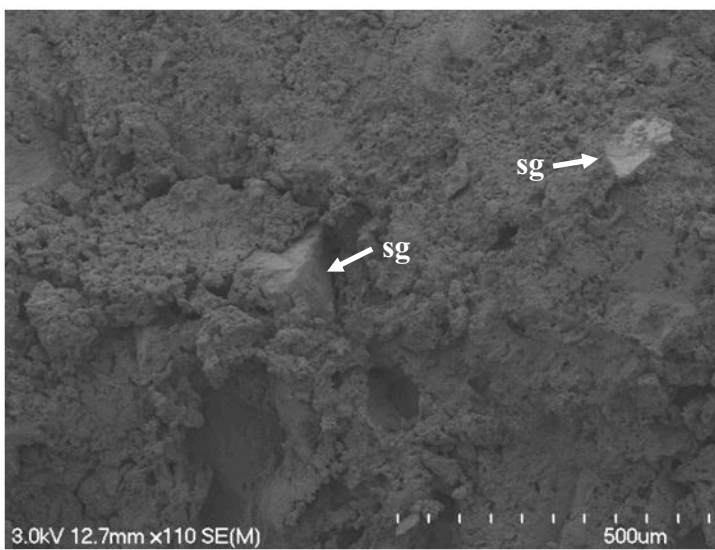
Figure 7.31: SEM image from OS4 displaying sand grains (sg) supported individually in a groundmass of clay size material. The sand grains appear embedded in the surrounding material with the groundmass lapping against the edges of the grains.
