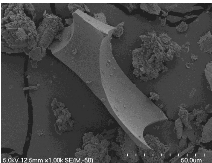
Figure 6.46: Volcanic glass fragment from Tauriko, the conchoidal fracturing represents bubble walls.
