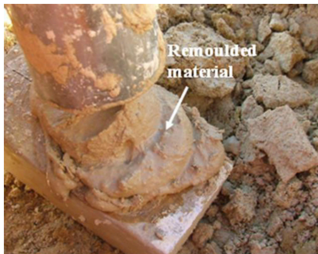
Figure 4.1: Remoulded clayey SILT (labelled) from Tauriko showing a dilatant character.
