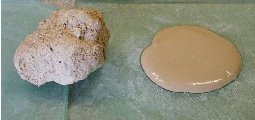
Figure 8.11: Sample TS1 before remoulding (left) and after (right). Peak and remoulded strengths are 57 kPa and 1 kPa respectively.
