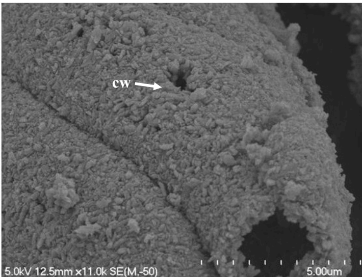
Figure 7.18: SEM image of a hollow tube from TS1. The opening of the tube is \sim 4 \mu\text{m} in diameter. The collapsed wall section at cw indicates the tubes delicacy.
