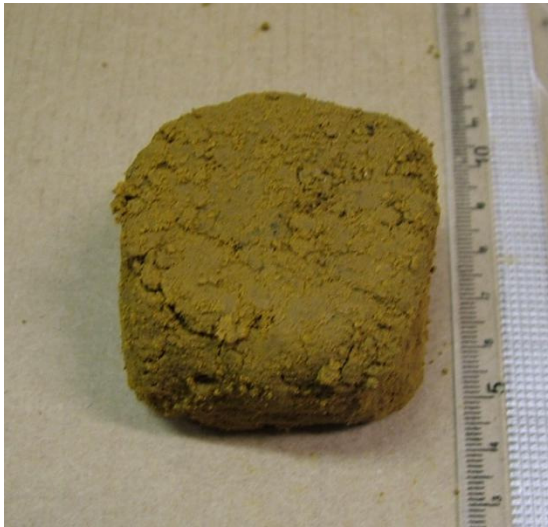
Figure 8.12: OS3 following remoulding. Remoulded strength is 36 kPa.
