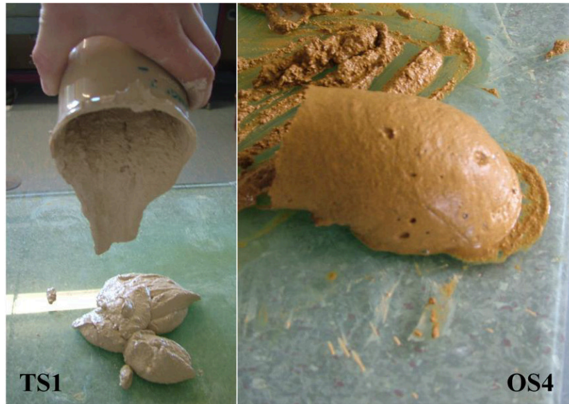
Figure 5.5: Remoulded UCS samples from TS1 (Tauriko) and OS4 (Otumoetai) displaying an inability to support cores because of extremely low remoulded strength. When tested with the shear vane both these samples had remoulded strength of < 2 kPa.
