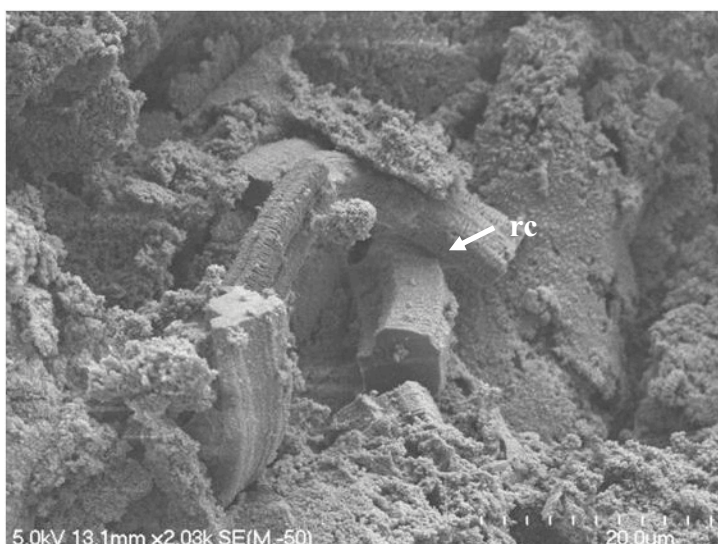
Figure 7.22: SEM images from TS3 showing books forming edge-to-edge right angle contacts (rc).
