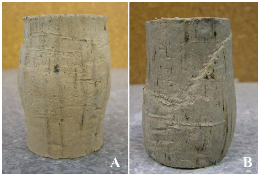
Figure 5.19: (A) Example of a barrel failure from TS1, \sigma_3 = 300 kPa, and (B) intermediate failure from TS3, \sigma_3 = 200 kPa.
