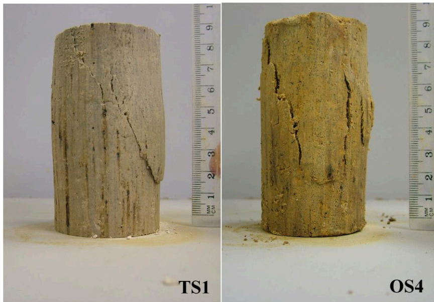
Figure 5.4: UCS samples from TS1 (Tauriko) and OS4 (Otumoetai) showing brittle type failure patterns. OS4 displays some vertical cracking to the right of the sample.
