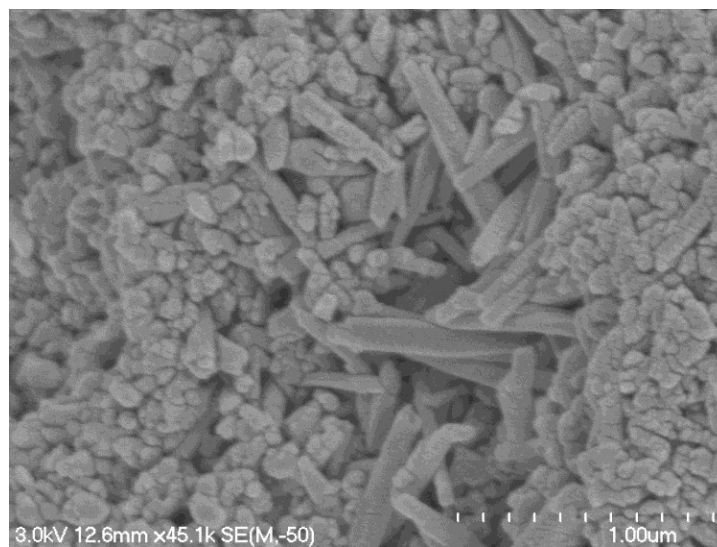
Figure 6.22: SEM image of material from OS4 (Otumoetai) showing very small ~0.1 \mu\text{m} irregularly shaped spheres. Many spheres appear to be either blocky or show an ovoid shape. Intermixed with the spheres is platy material of similar size. Tubes are present in the centre of the image and appear at least 0.8 \mu\text{m} long.
