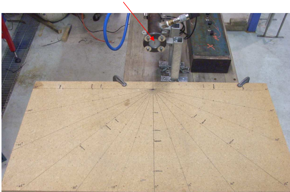
Figure 4.7, Orientation Board with markings for positioning of Ultraprobe.
