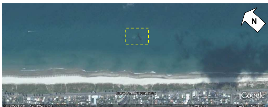
Figure 2.13. Satellite view of the Tay Street area at Mount Maunganui, New Zealand where the prototype reef was constructed (yellow square) dating from the 23/09/2006 (reef 70 % completed). Note the rhythmic bar and rip systems in the vicinity of the reef. (Source: Google Earth).
