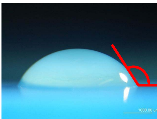
Figure 4.10: Example of air-PT water contact angle (4 minutes treatment time)
