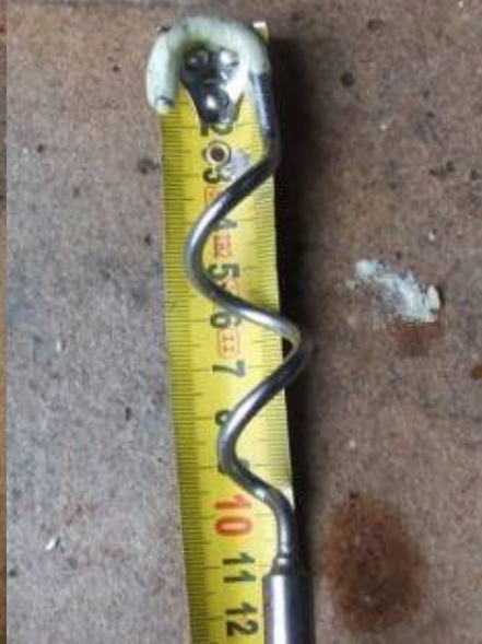
Figure 3.5: Mixing head showing size
