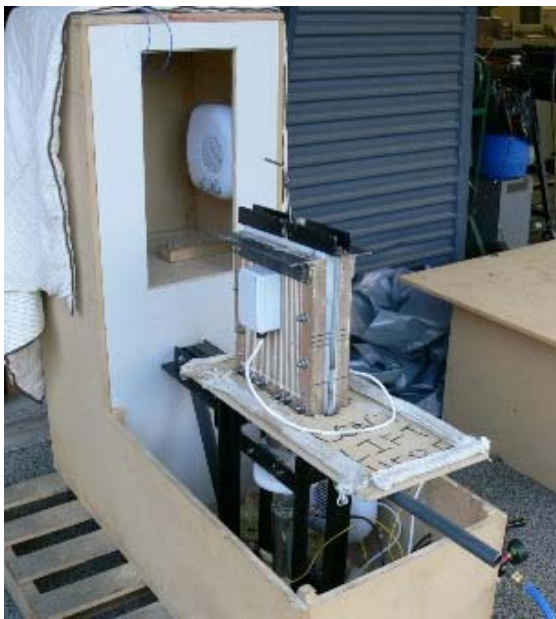
Figure 3.2: Foam processing - mould down
