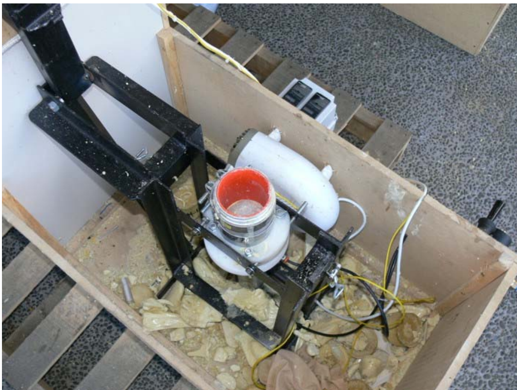
Figure 3.6: Mixing cup and equipment frame
