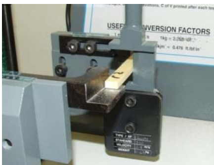
Figure 3.14: Impact tester anvil close-up
