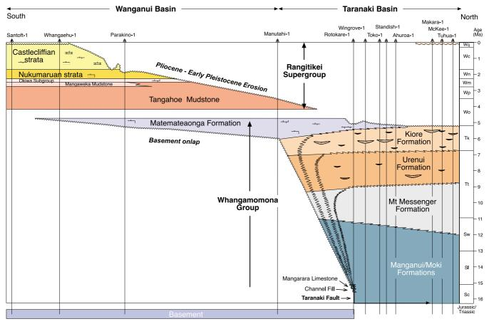
Fig.5. Wanganui Basin to Taranaki Basin (Santoft-1A to Tuhua-1) stratigraphic panel built up from well-to-well correlations, and related time-stratigraphic cross-section.
