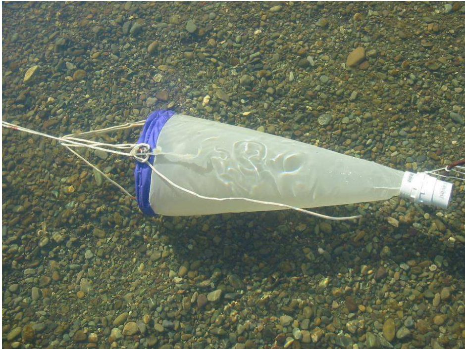
Figure A.1(19): Photograph of drift net used for sampling D. geminata . Taken from Cary et al. (2006).
