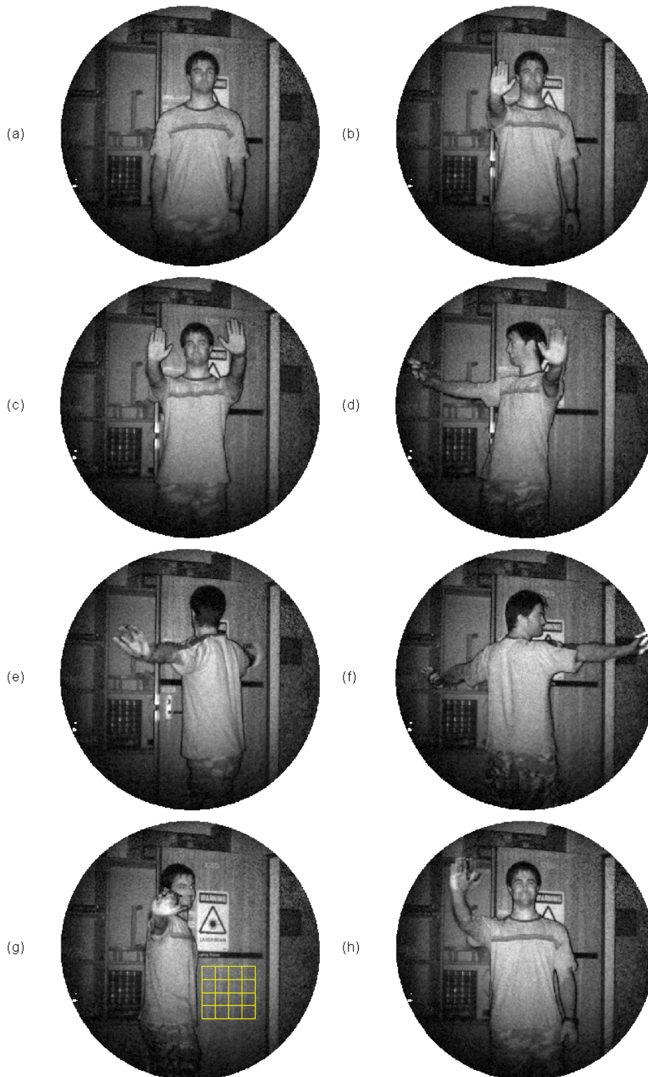
Figure 8.7: Selected intensity images of a moving person captured at a video update rate (25 fps). Corresponding range data are shown in Figure 8.8. Range precision is measured for the flat, bare region of the door in (g) for 25 \times 25 pixel segments illustrated by the grid pattern.
