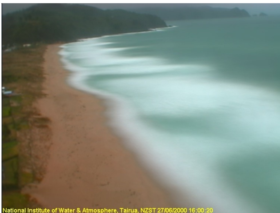
Figure 3.2. Un-rectified, time-averaged image (over a 15 minute duration) of Tairua Beach on Julian Day 179 at 0800 hours in 2000.
