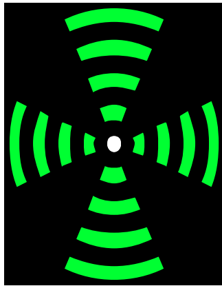
Figure 5-4. CorelDRAW X3 Graphic software layout design and the RGB colour scheme of an orthogonally paired selective polariton generator, plasmonic structure. The layout is scaled to the desired dimensions within the FIB milling software.
