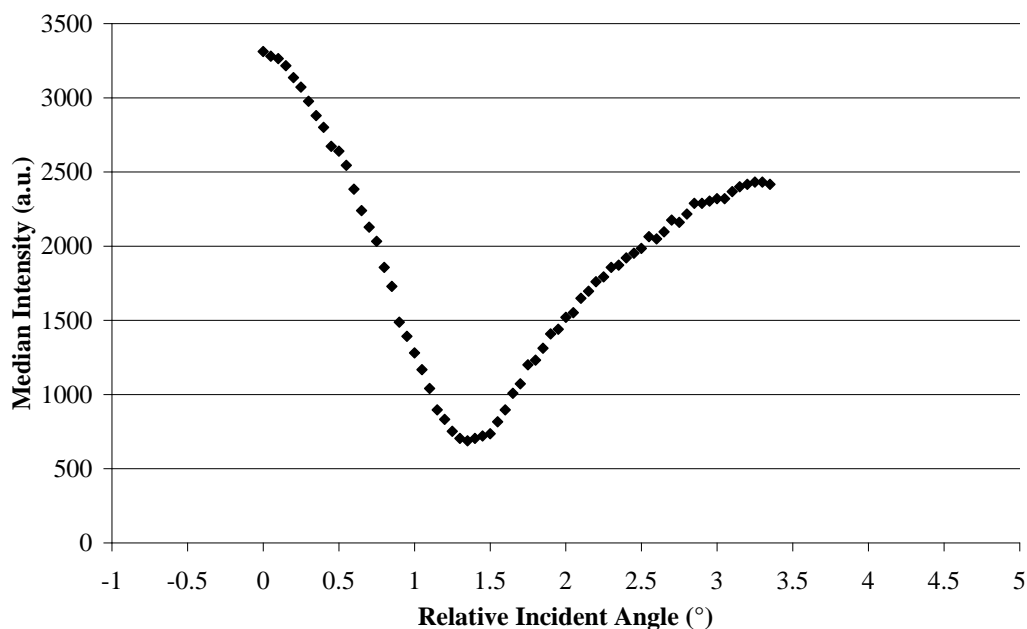
Figure 3-2. Intensity interrogation technique acquired SPR profile of the gold grating CD-R, illuminated with a 635 nm diode laser. The incidence angle was incremented by 0.05° steps, 3.35° around the resonance angle of 38°.
