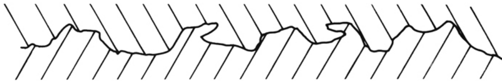
Figure 2.11: Schematic of mechanical interlocking [28].
