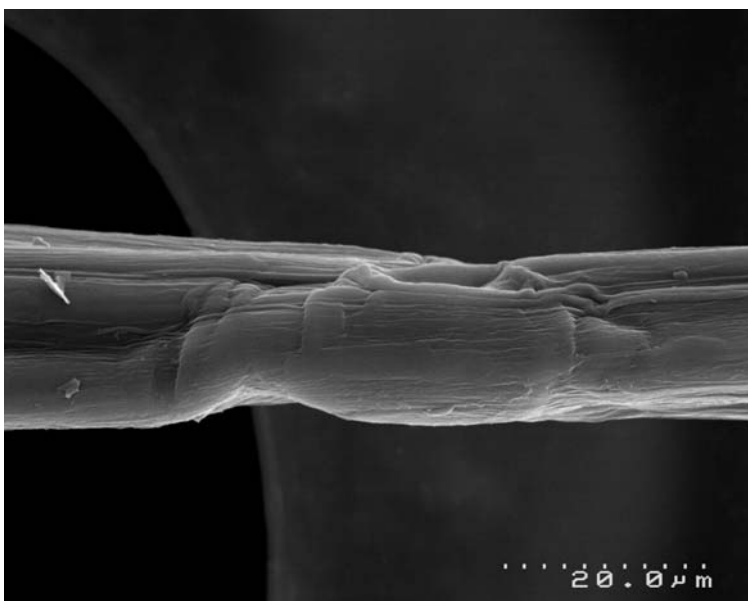
Figure 4.2.3: SEM of E treated hemp fibre
