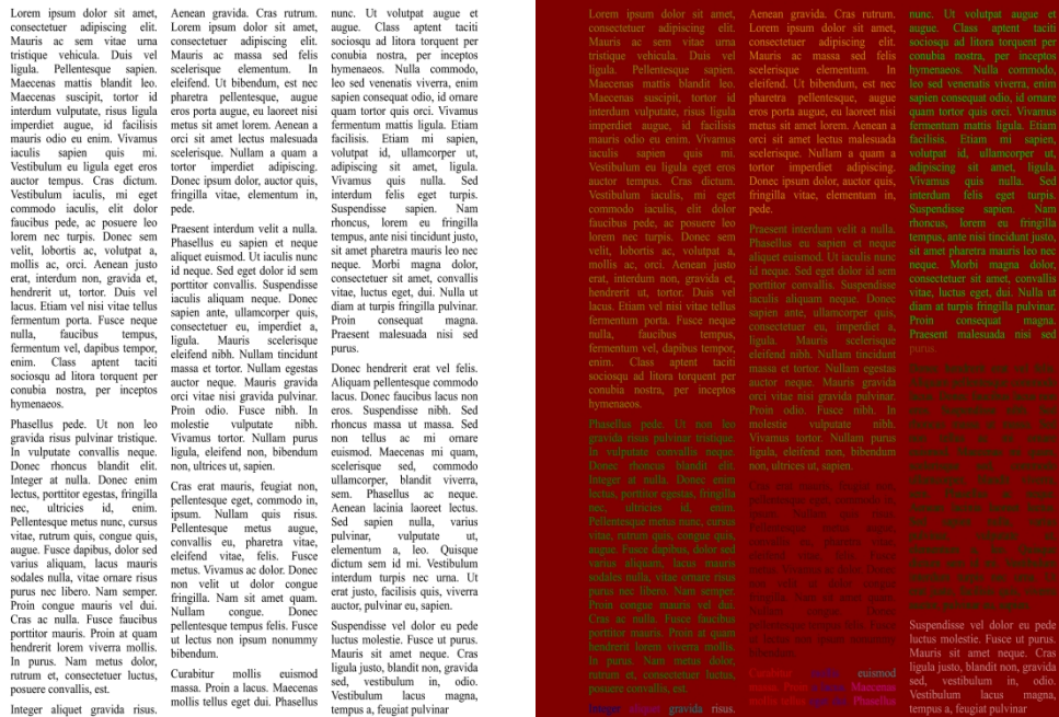
Figure 4.7: Example of XY-Cut segmentation on synthetic image (image dimension: 1700 x 2339, resolution: 96 DPI).
