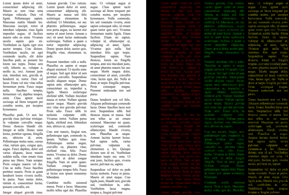
Figure 4.3: Example of RAST segmentation on synthetic image (column group, image dimension: 1700 x 2339, resolution: 96 DPI).
