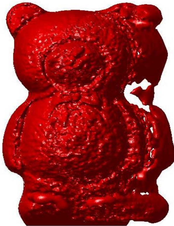
Figure 5.15 : Shape reconstruction using Fast RBF for two set of data ( 0^\circ and 30^\circ )
