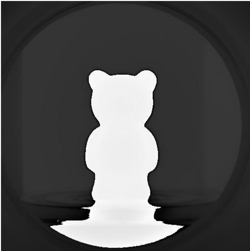
Figure 4.12 : Range image front view of bear captured from ranger camera
