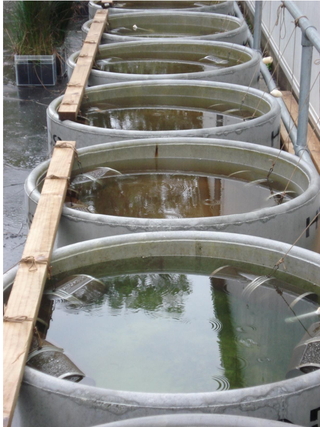
Figure 4.1 Gee minnow traps set in tanks at 400 mm water depth
