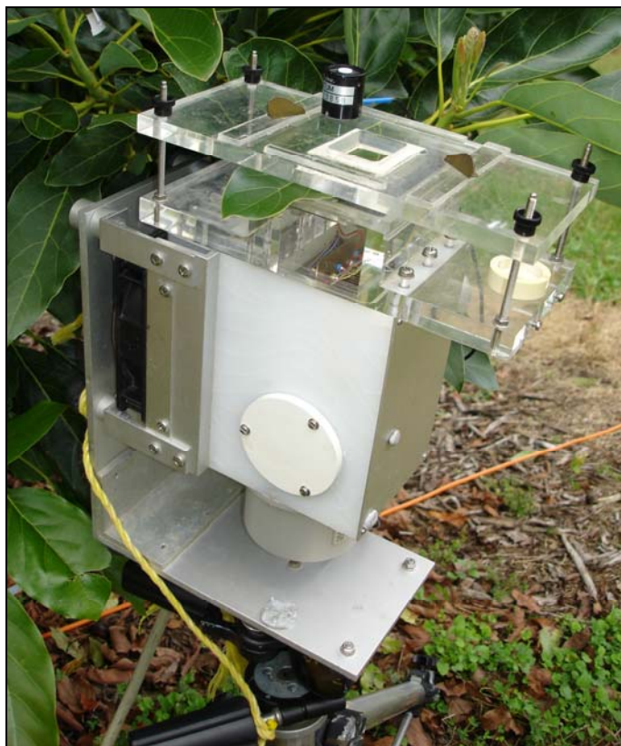
Figure 3.11 The climatized cuvette attached to the CMS-400.
