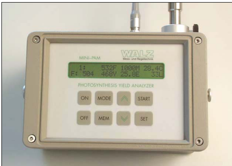
Figure 3.14 The Walz Mini-PAM photosynthesis yield analyser (Photo T.G.A. Green).
