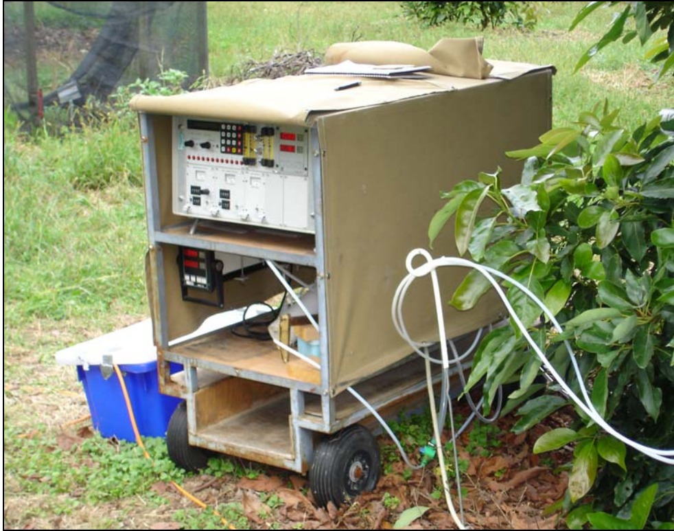
Figure 3.9 The CMS-400 mains powered, open flow, differential system for making continuous, automatic gas exchange measurements.
