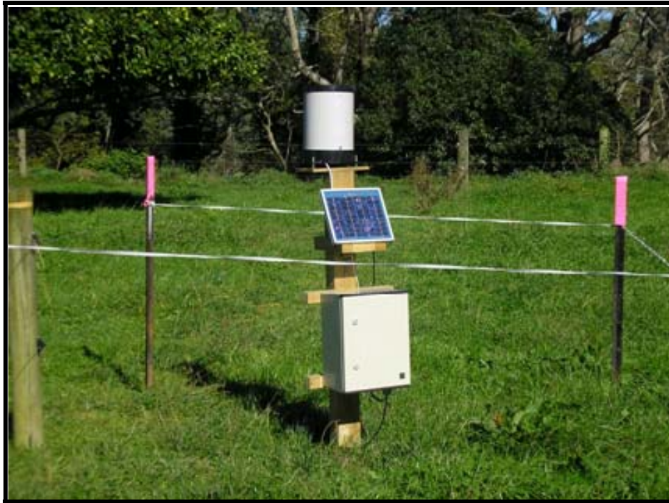
Figure 3.1 Time Domain Reflectometer set up at the field site at Dexcel's Scott Farm to measure soil moisture content and rainfall.
