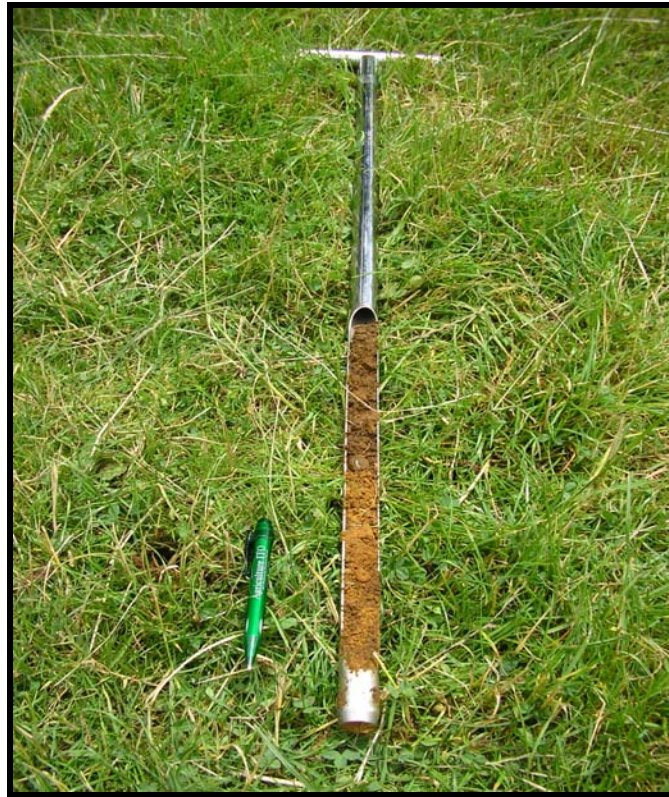
Figure 4.6 Soil sampler used to sample at different depths down the soil profile and to collect soil samples to measure the rate of DCD degradation
