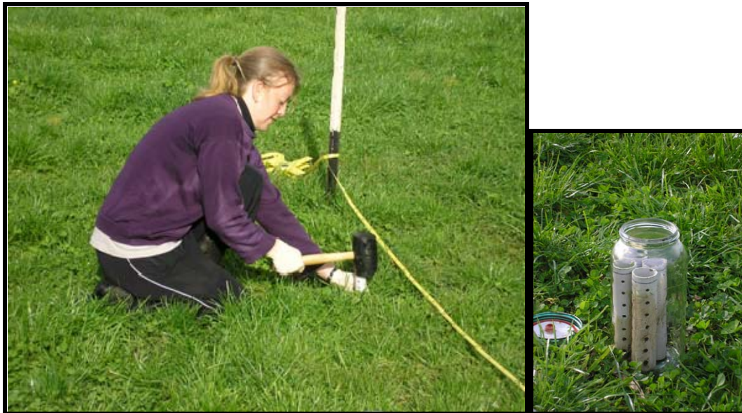
Figure 4.5 Field sampling to determine denitrification rates using the acetylene inhibition technique on intact soil cores (photos: Jacinta Parenzee).
