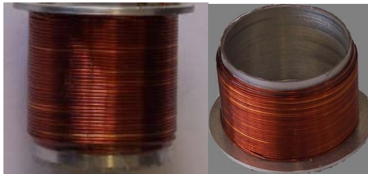
Figure 2-5 Aluminium bobbin with coil
