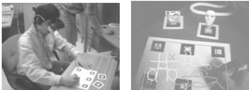
Figure 2.3: CSCW AR system. The left is a user who was doing the test with the system, The right is the image the user saw, which was drawn on the HMD
