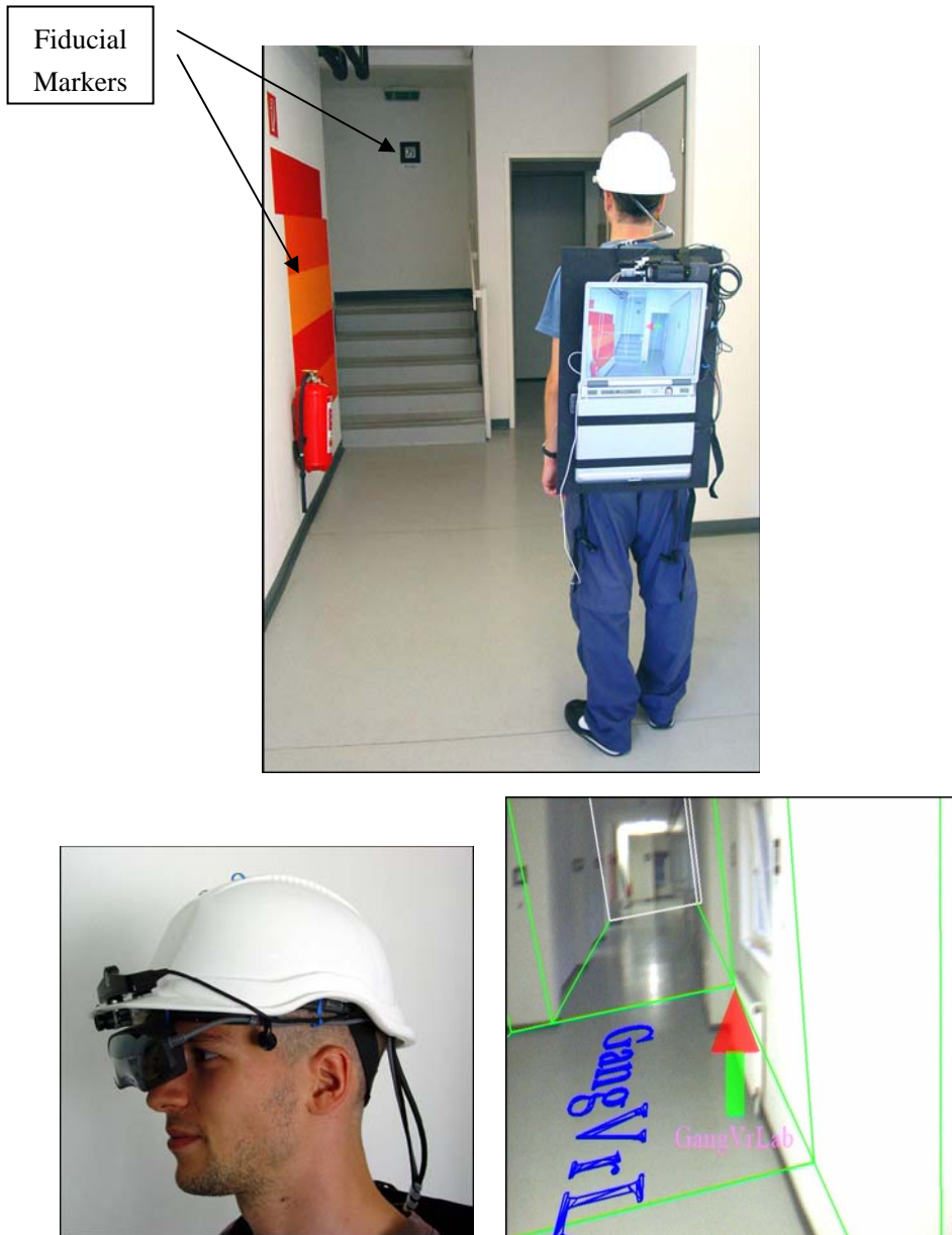
Figure 2.4: Location based Mobile AR system. The top shows the environment; the bottom left shows the HMD, helmet and the inertial sensor; the bottom right shows the image displayed in HMD
