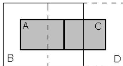
Figure 5.3: Our threshold algorithm. when converting area A to binary, area B will be used to calculate the local constant threshold value. Likewise, area D will be used to calculate the threshold for converting area C
