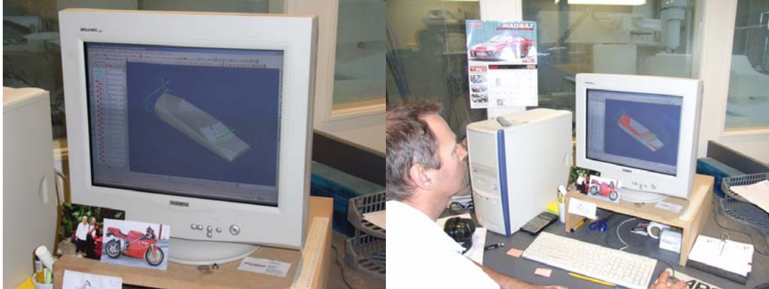
Figure 4.15 a) AlphaCam creating a cutting program b) An engineer simulates a virtual mill of the Ultracommuter body shell.
