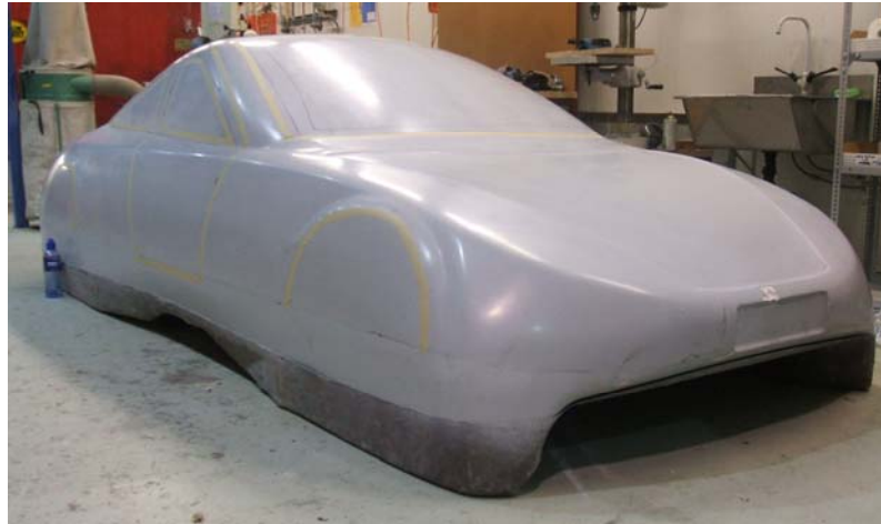
Figure 4.17 Plug after molds have been lifted with mocked shut lines on it
