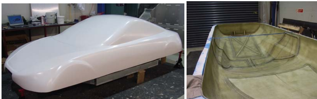
Figure 4.19 a) Ultracommuter body fresh from the mold b) Aluminium strengthening bars laminated in
