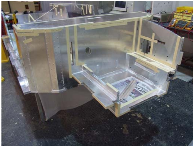
Figure 4.3 Aluminium honeycomb chassis under construction
