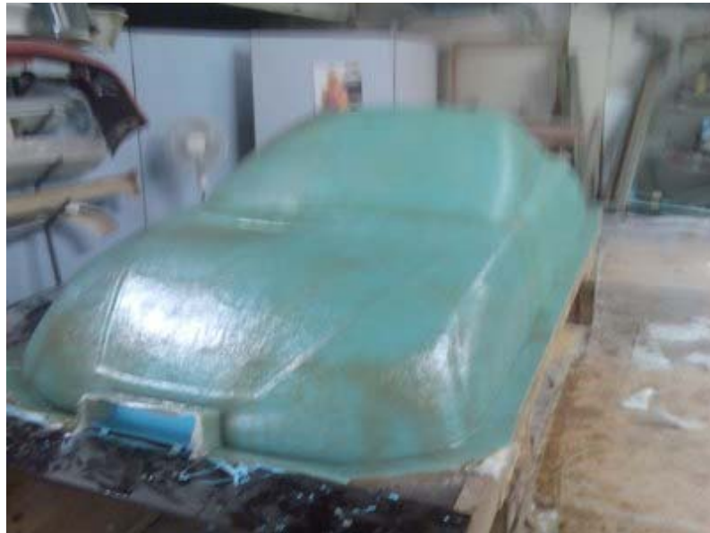
Figure 4.18 Ultracommuter mold, blue gelcoat coated by fibreglass layers
