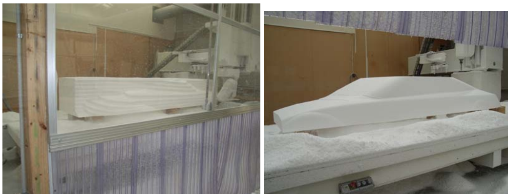
Figure 4.16 a) The 5-axis CNC creates a rough cut b) the finishing cut
