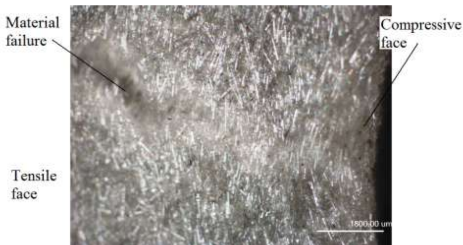
Figure 42. Failure shown on glass fibre composite bend sample.
