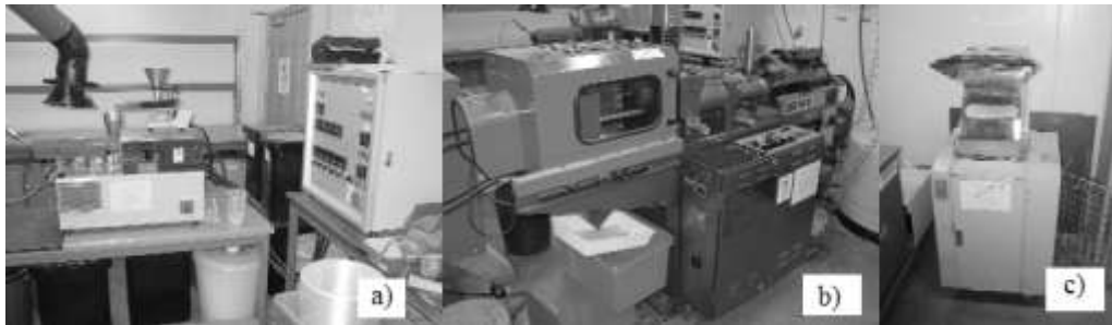
Figure A64. a) Thermo Prism TSE 16 TC twin screw extruder (TEX), b) Dr Boy 15kN Injection moulder (IM), c) Castin triblade granulator (CG).
