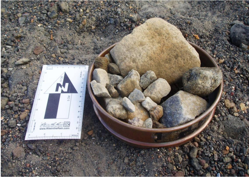
Fig. 3.1 >-4 phi grains removed from a matrix samples. 1.5 kg samples (weight of <16 mm fraction) were collected of diamicton matrix, >16 mm clasts were separated, measured and discarded in the field. A -4 phi sieve was utilised to remove the coarser fraction.
