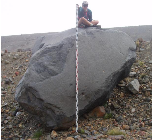
Fig. 3.2 Upper grain fractions of historic lahar deposits were measured in the field. A. A 25 m 2 grid for measuring outsized clasts (clasts greater than 6 cm in diameter) on historic lahar terrace surface (1975 deposit 7 km from Crater Lake). B. Maximum clast size measurement (3.46 m) in 1975 6.5 km from Crater Lake.
