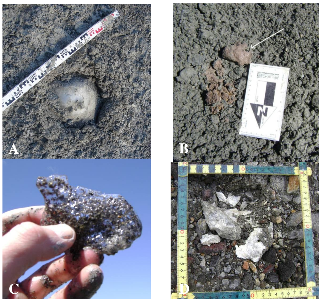
Fig. 5.15 Components unique to the 2007E flow. A. Perennial snow blocks, up to 25 cm, occur in the second of the major concentrated pulses near the surface of the deposit. The snow had coarser crystal sizes than the matrix of seasonal snow. B. Flaky clasts up to 6 cm in diameter of lake mud that remould rapidly when disturbed. The arrow indicates remoulded clast. Arrow 10 cm. C. Clast of clear ice occur in first pulse, lower unit, of 2007E. Approximately 6 cm across. Photo: Michael Tayler. D. Accumulation of gypsum on hydrothermally altered clast. Divisions on scale are 10 cm.
