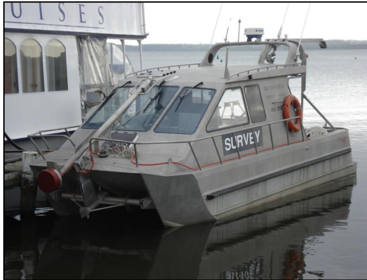
Figure 4.1. The 9 m catamaran “Tai Rangahau” has a bow mounted MBES, and stern mounted SBES. The vessel was purpose built as a surveying and diving vessel.
