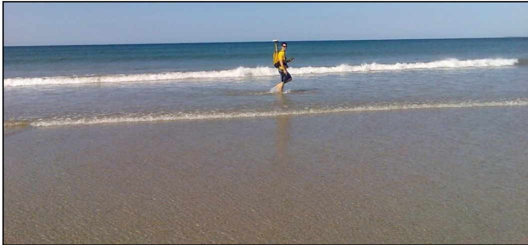
Figure 4.20. Topographic survey of intertidal and dry beach (high water to toe of dune) using backpack mounted RTK GPS.
