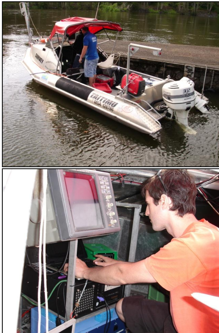
Figure 4.2. The 6 m Pontoon vessel, “Taitimu”, is a multi-task craft with a bow mounted MBES and a stern mounted SBES.
