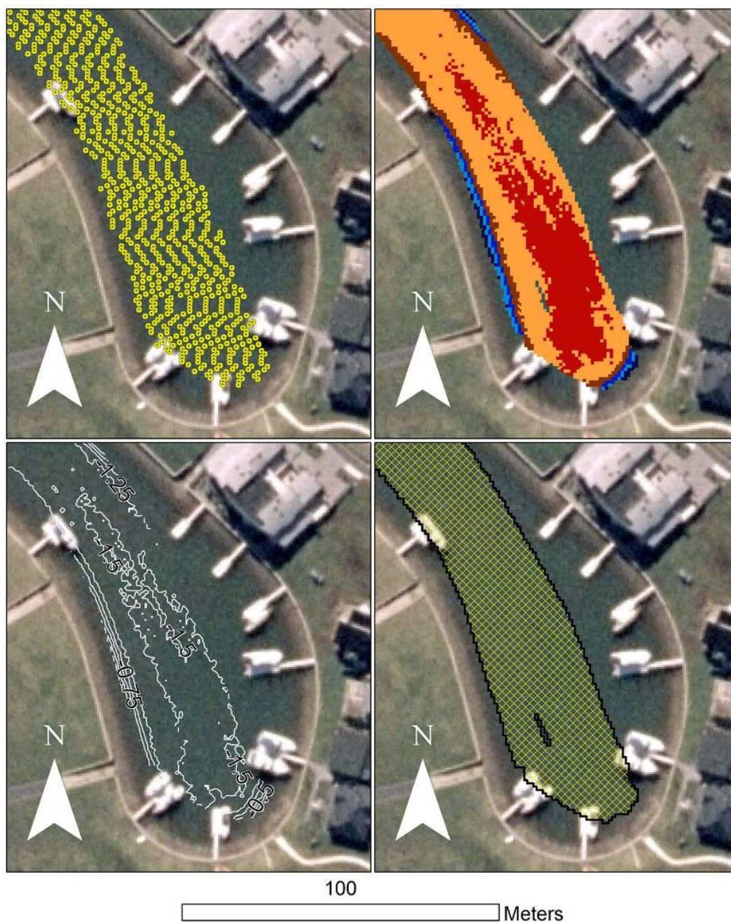
Figure 5.6. Images of geodatabase MBES data products for a canal development in Whitianga (New Zealand). Clockwise from top left: SoundingPoint feature class, cell-based raster, sounding coverage and contours. The soundings are filtered to display only every 5 th point, and this can be set to vary with viewing scale using “Layer” settings.
