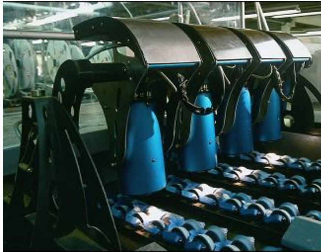
Figure 1.2. Multi-lane near infra-red (NIR) grading system (Taste Technologies Ltd, Auckland, New Zealand) fitted to a commercial kiwifruit grader (Compac™ grading equipment, Auckland, New Zealand).
